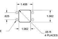
BOTTOM MOUNT-CLEARANCE HOLE FOR .192 SCREW TOP MOUNT-CLEARANCE HOLE FOR .112 SCREW
